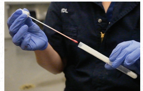
6. Place the swab into a labeled, sterile tube. Promptly refrigerate samples for shipment and submit to a veterinary diagnostic laboratory.
